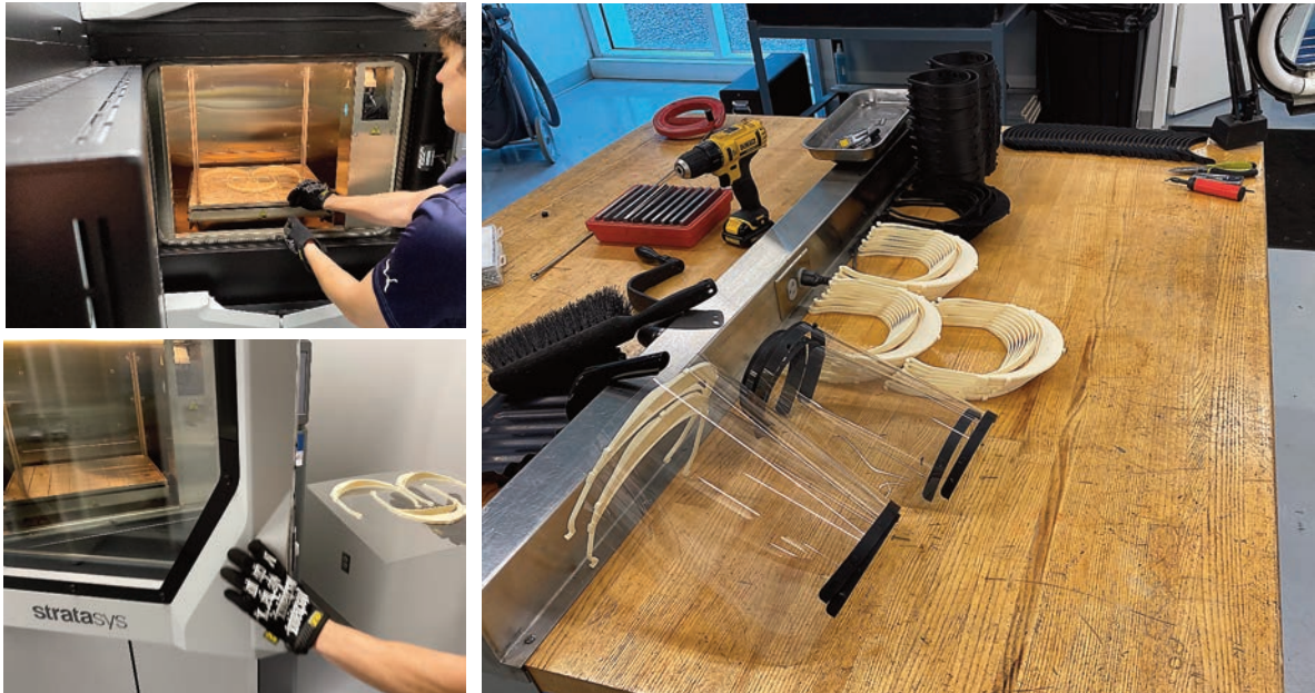
3-D printers at NASCAR's Research & Development Center in Charlotte produced thousands of protective face shields that were shipped across the country.
